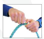
3. Ensure that tab will stay perpendicular to the belt's running direction; reverse the belt upside down to let it run on the tab side.
