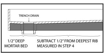
5. Turn the shower pan over and note that there are ribs under the shower pan floor. To calculate the amount of mortar needed, you will need to know the depth of the deepest point in between the ribs. Once you have that value, calculate the thickness (depth) of your mortar base (Type N or S Mortar) using the following formula:
