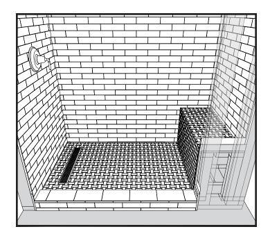
15. Adjust the height of the drain as necessary to accommodate the floor covering. Set your tile using a white modified thin-set/tile mortar and a notched trowel as specified by the thin-set/tile mortar manufacturer based on your tile size. Tile Redi recommends the modified thin-set/tile mortar products found in table below.
