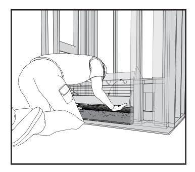
9. Place the pan in the mud base and firmly but gently shimmy the pan (applying pressure in drain location first) into the mud so that (i) the drain is fully supported by mud at the bore hole in the substrate, and (ii) the ribs are completely filled with the mud alternately applying hand pressure to the right and left sides of the pan floor until the pan ribs come within 1/8" clearance of the subfloor.
