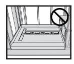
11. Install the Redi Flash flashing system along the splash walls of the shower pan. Apply a bead of 100% silicone to the top of the Redi Flash flashing that runs along the splash wall alongside the bench frame.
