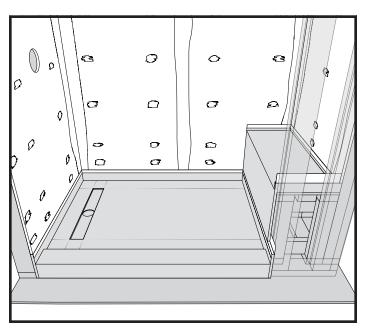
14. Install the shower backer board and waterproofing in accordance with the standards established by the Tile Council of North America, Inc. Seal and waterproof joint between backer board and the shower pan splash walls using Redi Flash® or 100% silicone. It is recommended to use a membrane and fluid applied waterproof in addition to the Redi Flash® or 100% silicone.
