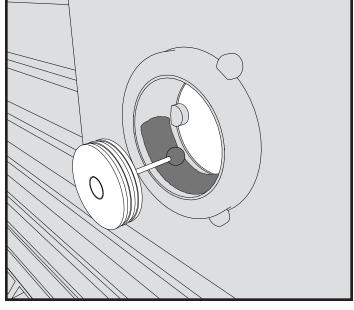
If there is no access from the subfloor below and you followed step 3b, then brush primer and PVC adhesive on the drain pipe stubbed up from the subfloor, then quickly insert the stubbed-up drain pipe properly into the shower pan drain.\*\*
