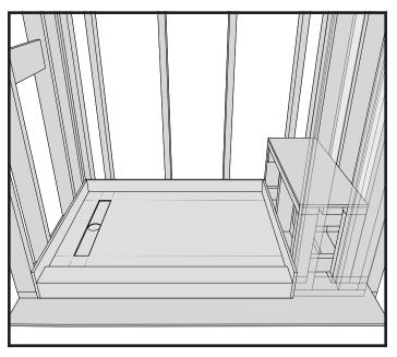
3. To ensure a perfect fit, test fit shower pan drain housing into subfloor bore hole. Make sure the shower pan is aligned properly and fits snuggly against the shower frame studs on all sides and corners. Ensure that the pan is level on the floor. There should be no movement or bulge.
