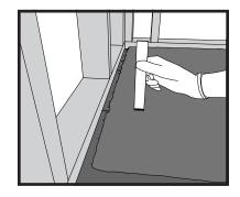
8. If there is access from the subfloor below and you followed Step 3a, then brush primer and PVC adhesive on the inside of the drain and outside of the cut drain pipe and quickly insert into drain connection, then be sure the drain pipe extends far enough below the subfloor so it can be connected to the waste water pipe following the installation.
