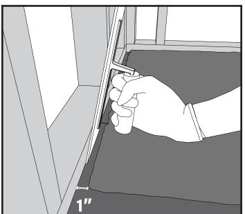
7. Offset the mortar base 1" from each outside edge of the pan with exception of the curb side. Mortar will protrude out from under the curb, run the finishing trowel along curb face to backfill any excess mortar.
