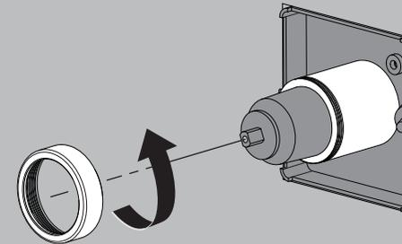
**3** Clean front surface of wall. Ensure that the Delta Valve Stops (3) are in the open position by unthreading Valve Stop counter-clockwise. Install Valve Mounting Plate (1) to existing Delta Valve, using the 10-24 x 1-1/2" screws (2) provided. Take care to not over tighten mounting screws or damage may occur.
