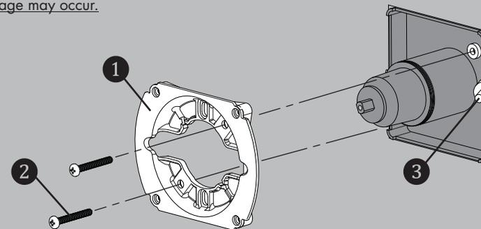
**NOTE:** Depending on the mounting depth of the Delta Valve, the Valve Mounting Plate (1) may contact either the surface of the wall, or the Plaster Guard of the Delta Valve when secured into the final position.
