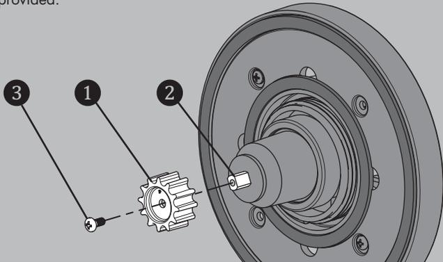
7 Orient the Decorative Wall Plate (1) as shown below and insert the RED index button into the top hole of the Wall Plate, and the BLUE index button into the lower hole. Slide Wall Plate Assembly over Wall Mounting Plate (2).
