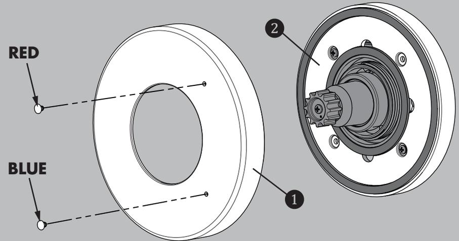
8 Orient the Handle Assembly in a vertical position as shown below. Guide Handle Assembly onto the Spline Adapter (3). While holding the Handle (1) stationary in the vertical position, thread the Handle Escutcheon (2) onto the Wall Mounting Plate (4). Hand tighten until snug.
