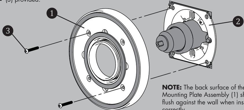
**NOTE:** The back surface of the Valve Mounting Plate Assembly (1) should sit flush against the wall when installed correctly.
