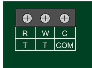
R, W, C and T, T, COM dual labeling at thermostat terminals. Compatible with low voltage 2, 3, or 4 wire thermostats or any other low voltage devices having a switching action.
