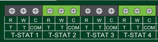
When a zone has a demand from a thermostat (TT/RW) the control will send 120 VAC to the corresponding zone pump, primary pump and the (X X) dry contact will close to signal the boiler of a heating demand. AUX
