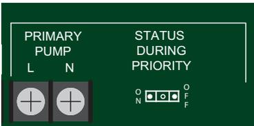
**Status During Priority ON / OFF:** When status jumper is placed on the ON pins, the primary pump will continue to operate during ZONE 1 priority demand. When jumper is placed on the OFF pins, the primary pump will be OFF during ZONE 1 priority demand.
