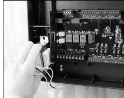
Slide bottom end of transformer into bottom latch.
