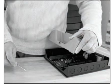
**Mounting:** Do not mount to a surface that exceeds 115°F (45°C). The unit must be only located in dry interior locations. Use only copper conductor supply wire suitable for at least 105° C. All circuits must have a common disconnect and be connected to the same pole of the disconnect. It is not suitable for installation in hazardous locations.
