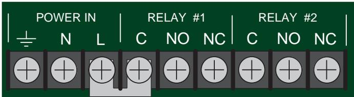
If dry contacts are desired from relay #1, remove the factory installed jumper between L and C.
