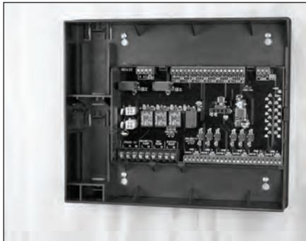
Mount box on stable surface using level.
