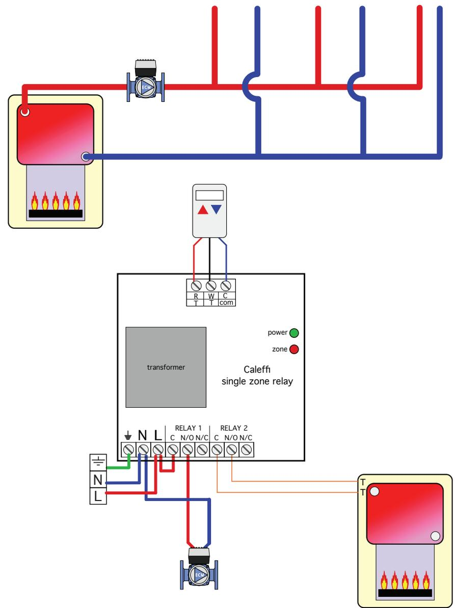
Hydronic diagram is for illustration purposes only, some components have been removed for simplicity.
