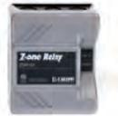
The ZSR101 is a versatile single relay control with two outputs for operating a 120 VAC pump with boiler enable, or two 120 VAC devices without boiler enable. Features include rear knock outs for 4x4 junction box mounting, convenient pre-installed jumper for pump operation, and 10 amp total load rating.
