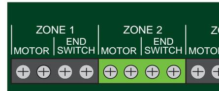
Motor = 24 VAC to power the zone valve motor
