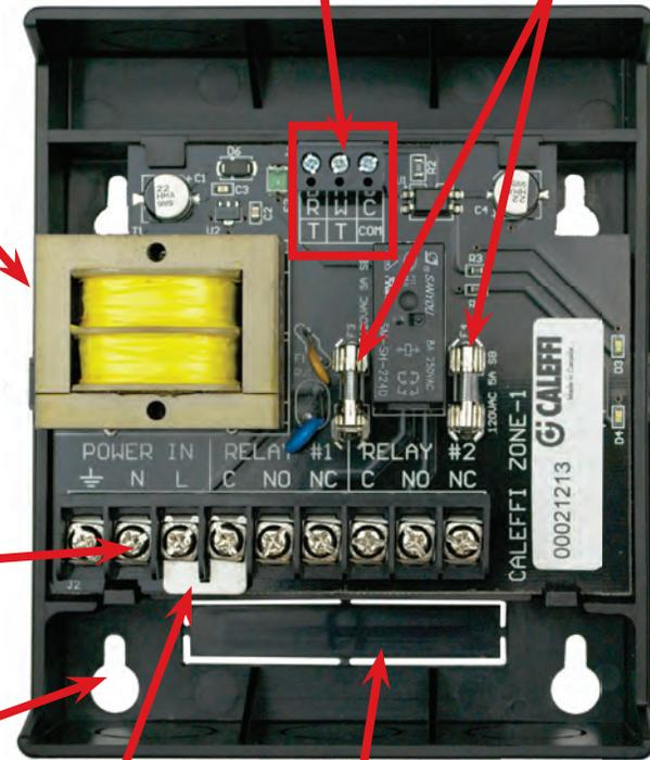
**Mounting:** Do not mount to a surface that exceeds 115°F (45°C). The unit must be only located in dry interior locations. Use only copper conductor supply wire suitable for at least 105° C. All circuits must have a common disconnect and be connected to the same pole of the disconnect. It is not suitable for installation in hazardous locations.
