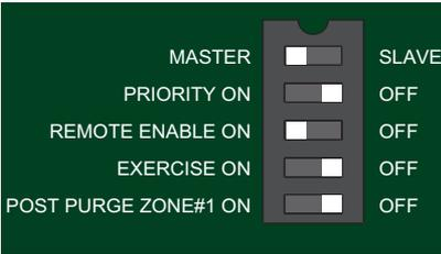
The ZSR series of control is programmed by positioning five dip switches for the following operations.
