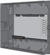
Remove cover of relay box. Identify the four mounting holes on relay box, mark on the wall the desired location of mounting. Drill, anchor, and fasten four screws for mounting.
