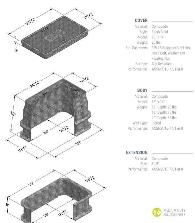
For use in non-vehicular traffic situations only. Weights and dimensions may vary slightly. Actual load rating is determined by the box and cover combination.
