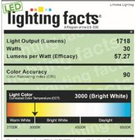
All results are according to IESNA LM-79-2008: Approved Method for the Electrical and Photometric Testing of Solal-State Lighting. The U.S. Department of Energy (DOE) verifies product test data and results.
