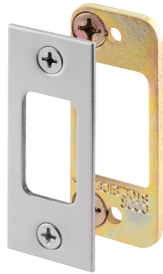
Qty: 1 set, with fasteners. 1/8 in. thick heavy gauge steel base, 2-1/8 in. hole spacing, improves security with 3 in. long screws attaching to wall stud. E 2479 (Brass finish) E 2482 (Bronze finish) E 2480 (Antique brass finish) E 2688 (Stainless steel) E 2483 (Satin nickel finish) E 2796 (Matte black finish)
