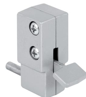
Qty: 1, with fasteners. Diecast housing, hardened steel bolt, foot operation, 5/8 in. projection, 5/8 in. hole spacing. U 9877 (Aluminum finish) U 9879 (White) S 4041 (Black)
