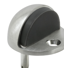
Qty: 1, with fasteners. Cast brass housing, rubber bumper, 15/16 in. hole spacing, floor mounted, meets ANSI standards.
