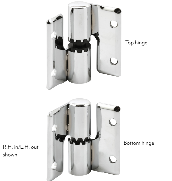
Qty: 1 set, with fasteners. Top and bottom, surface mounted, 1-1/2 in. hole spacing. 658-6575 (Chrome plated brass – R.H. in/L.H. out) 658-6572 (Chrome plated brass – L.H. in/R.H. out)
