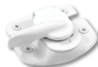
Qty: 1 set, with fasteners. Stamped steel, cam action, 1-3/4 in. hole spacing. U 9924 (Brass finish) U 9925 (White) U 11062 (Satin nickel finish)
