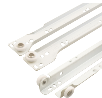
Qty: 2 sets, with fasteners. Steel track, left and right hand, 3/4 in. O.D. plastic roller. R 7210 (15-3/4 in. length) R 7212 (19-3/4 in. length) R 7211 (17-3/4 in. length)
