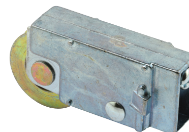
Qty: 1 Diecast housing assembly, end adjustable, 1-1/4 in. O.D. steel ball bearing roller, center grooved.
