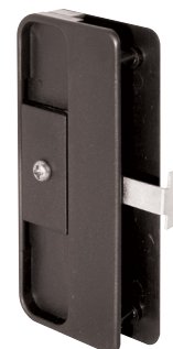
Qty: 1, with fasteners. Plastic inside and outside handles, steel latch, 3-1/4 in. hole spacing, non-handed. A150 (Black)
