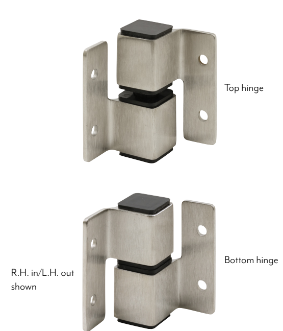
Qty: 1 set, with fasteners. Square barrel, top and bottom, surface mounted, 1-1/2 in. hole spacing. 658-2019 (Satin cast stainless steel – R.H. in/L.H. out) 658-2022 (Satin cast stainless steel – L.H. in/R.H. out)
