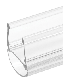
Qty: 1 Clear vinyl, “Bulb” vertical side seal, 78 in., UV resistant, mold resistant with anti-fungal additives. M 6322 (Fits 1/4 in glass) M 6323 (Fits 3/8 in glass) M 6324 (Fits 1/2 in glass)
