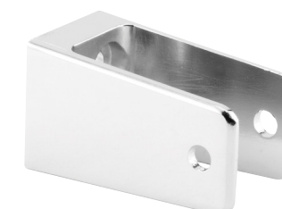
Qty: 1, with fasteners. "U" bracket, for 1-1/4 in. thick panels, 2-1/2 in. length. 656-6428 (Chrome plated zamak)
