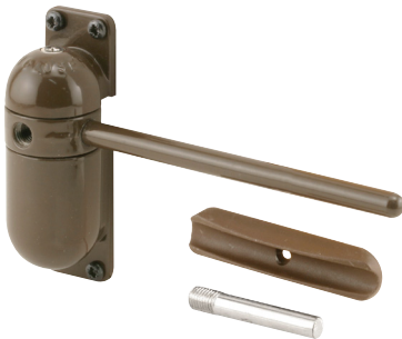
Qty: 1, with fasteners. Diecast zinc body incorporates one torsion spring, adjustable, weather resistant, non-handed, for doors and gates up to 57 lbs. KC50HD (White) KC57US (Brown)
