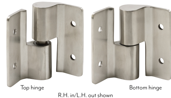
Qty: 1 set. Top and bottom, surface mounted, all metal inserts, 1-1/2 in. hole spacing, satin cast stainless steel.
