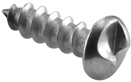
One-way sheet metal screw. 642-0618 (#10 x 1/2 in., Stainless steel, Qty. 100) 658-0358 (#10 x 5/8 in., Stainless steel, Qty. 50) 651-0358 (#10 x 5/8 in., Chrome plated steel, Qty. 100)
