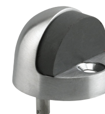
Qty: 1, with fasteners. Cast brass, 1 in. hole spacing, 1-5/16 in. height, 1-11/16 in. O.D. base. 658-1030 (Brushed chrome) 658-1027 (Satin nickel)
