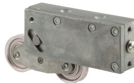
Qty: 1 Diecast housing assembly, end adjustable, 1-1/2 in. O.D. tandem ball bearing rollers, center grooved. D1586 (Steel) D1884 (Stainless steel)
