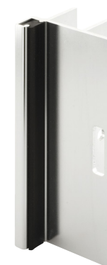
Qty: 1 Inswing for slide latch, for 1 in. thick square edge posts, 2-1/2 in. hole spacing. 658-2873 (Clear anodized extruded aluminum, no fasteners ) 656-4046 (Brite dip extruded aluminum, with fasteners )
