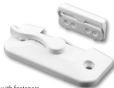
Qty: 1 set, with fasteners. Diecast, 2-1/4 in. hole spacing, cam action, 1/2 in., 3/4 in. and 1 in. keeper hole spacing. F2899 (White)
