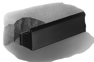
Cutaway from street, showing curb guard.
