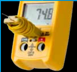
Type K Thermocouple Plugs Directly into Meter (SC240/SC260)
