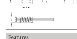
Elgen's Spring End Bearing is used conjunction with damper blade or controlling the damper inside the ductwork.
