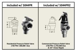
**Specifications:** Designed for residential or commercial use with potable water. This approved Webstone valve features an adjustable packing gland. Solder joint temperature ratings are per ASME B16.18 Annex A for 95-5 solder. Other solder materials have lower pressure/temperature limits. Do not silver braze or over heat valves when soldering.
