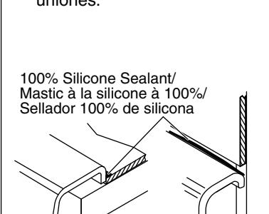
**12** Install the finished wall and deck material to within 1/16" (2 mm) of the bath rim.
