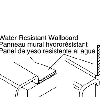
**11** Apply a 1/8" (3 mm) bead of 100% silicone sealant along the seams.
