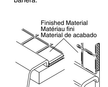
**13** Apply 100% silicone sealant around the bath along the finished walls and deck.
