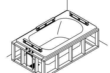
**8** Apply weight to the bath basin until the mortar or adhesive sets.
