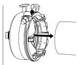
**Step 4** • With the bolt in the extended position, place the end cap onto the pipe end until the pipe makes contact with the inside of the end cap. **Note:** If it's impossible to bottom-out the pipe, ensure there is a minimum of 4" of pipe insertion.
