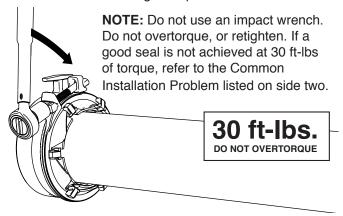
**Step 7** • Confirm proper installation by pressurizing the line and checking for leaks.
