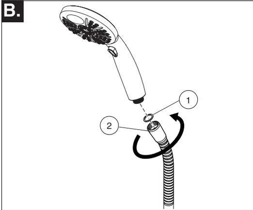
**A.** Ensure gasket (1) is inserted into the hose (2). Connect the hose to your designated water supply.
