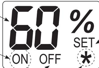
**SET** is displayed when ▲ or ▼ is pressed. The value displayed is the humidity setting. See **FIGURE 5**.
