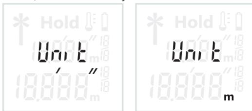
Switch off the measuring tool. Press the measuring button **1** and hold it down. The display will alternately show both units of measure. When the desired setting is displayed, release the measuring button 1. The setting is saved.
