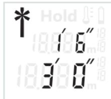
Press the "HOLD" button **1** once more to switch the laser on again. The laser indicator
