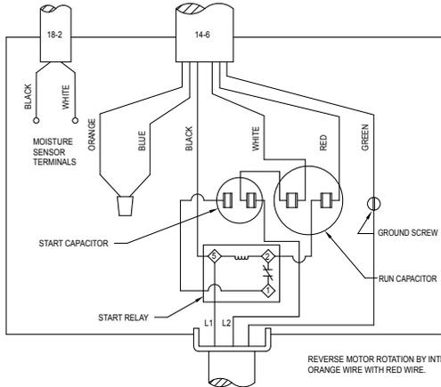
REVERSE MOTOR ROTATION BY INTERCHANGING ORANGE WIRE WITH RED WIRE.
