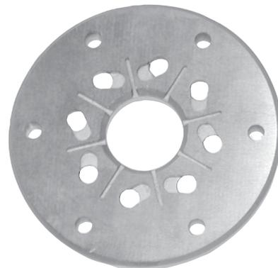
Grind the Star Cutter and Disc seen here to a 32 microfinish. Surfaces must be flat to within 0.001" T.I.R. Gap must be between 0.004" and 0.008" on these parts.
