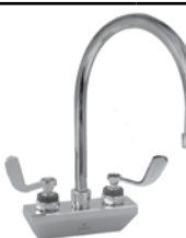
4" (102mm) Wall Mount with 8" (203mm) Swivel Gooseneck Spout and 4" Wrist Blade Handles
