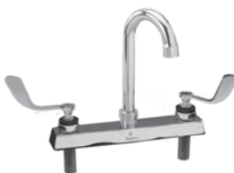
8" (203mm) Deck Mount with 3-1/2" (89mm) Swivel Gooseneck Spout and 4" (102mm) Wrist Blade Handles
