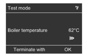
Emissions test mode should only be activated by your flue gas inspector during the annual inspection.
