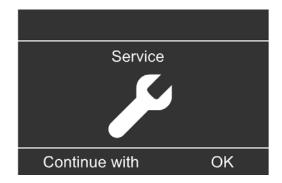
If your heating system is due for a service, the symbol \*Fflashes in the display, and "Service" appears.
