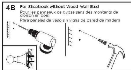
**4B** For Sheetrock or Ceramic tile Installation: drill 3/16" holes, be sure to keep drill level. Insert anchors into drilled holes using a hammer to tap the anchors in. Be careful not to break tile.
