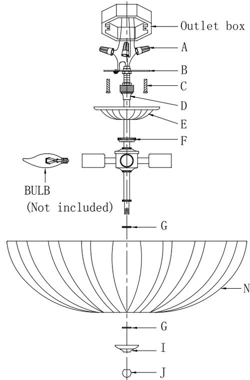
1. Install the crossbar (B) with ceiling loop (D) to outlet box by using mounting screws (C) provided.
