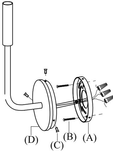
1. Remove mounting plate (A) from fixture base (D) by removing base screws (C).
