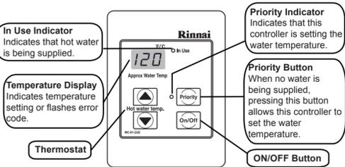
**WARNING** MC-91-1, MCC-91-1, MC-100V-1, and BC-100V-1 controllers are not compatible with Alternate Temperature Settings. Alternate Temperature Settings are for commercial applications only. DO NOT use the MC-91-1, MCC-91-1, MC-100V-1, or BC-100V-1 controllers when dip switches 2 and 3 (Dip SW2) are in the ON position.
