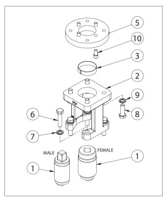
Figure C Linkage Assembly – Square Drive
