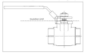
Figure 5 Insulation Limit
