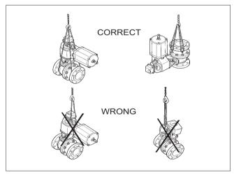
Figure 2 Lifting the valve
