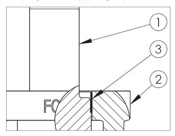
Figure B Proper Bearing Location
