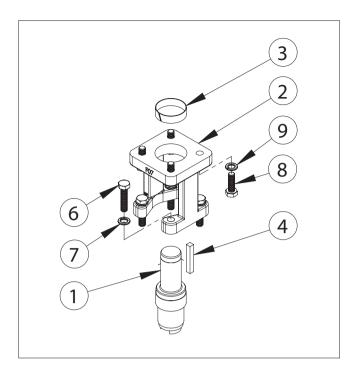
Figure A Linkage Assembly - Key Drive
