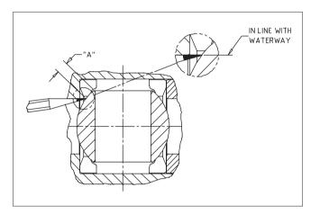
Figure 17. Correct Ball Position
