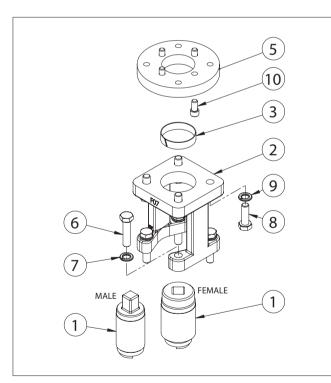
Figure 16. Linkage Assembly – Square Drive
