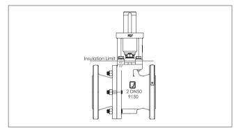
Figure 4. Insulation of the valve
