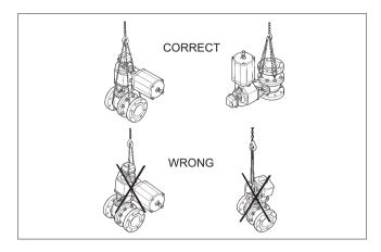
Figure 2. Lifting the valve
