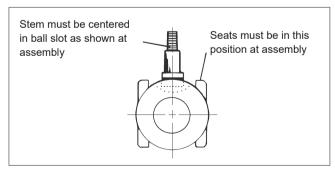
Figure 6. Proper Seat and Ball Orientation
