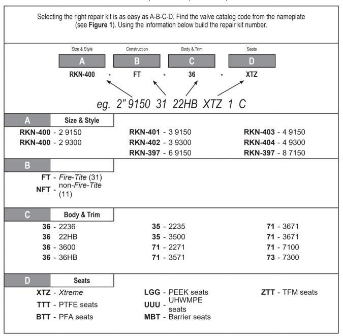
**WARNING:** If the valve you are selecting a Repair Kit for has a "Special Service" tag, check with your authorized Neles Distributor for help in selecting the correct kit.
