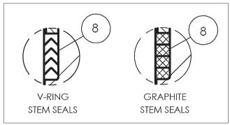
Figure 8. Stem Seal Orientation
