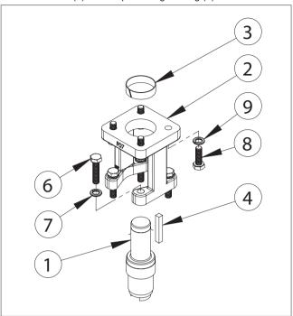
Figure 14. Linkage Assembly – Key Drive
