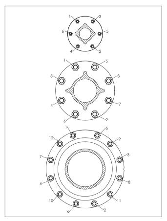
Figure 10. Bolt Tightening Sequence
