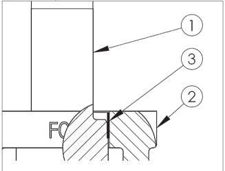
Figure 15. Proper bearing locations
