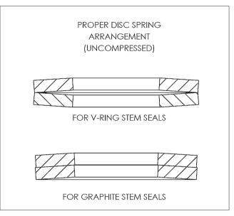
Figure 9. Disc Springs Orientation
