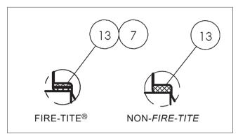
Figure 7. Thrust Bearing Orientations
