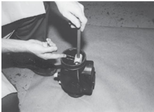
7. Insert the torsion spring and tool into the valve body. Position the coils between the ears of the disc in alignment with the shaft holes. While continuing to hold the tool, release the tongue of the torsion spring so that it presses against the center of the disc without unwinding.
