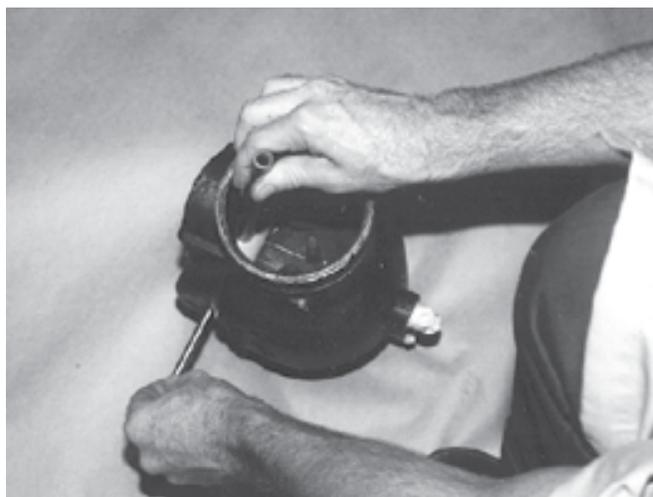
8. While holding the tool with one hand, insert the new shaft (provided in the kit) into the valve. Pass the shaft through the disc, torsion spring, and into the other side of the valve body.
