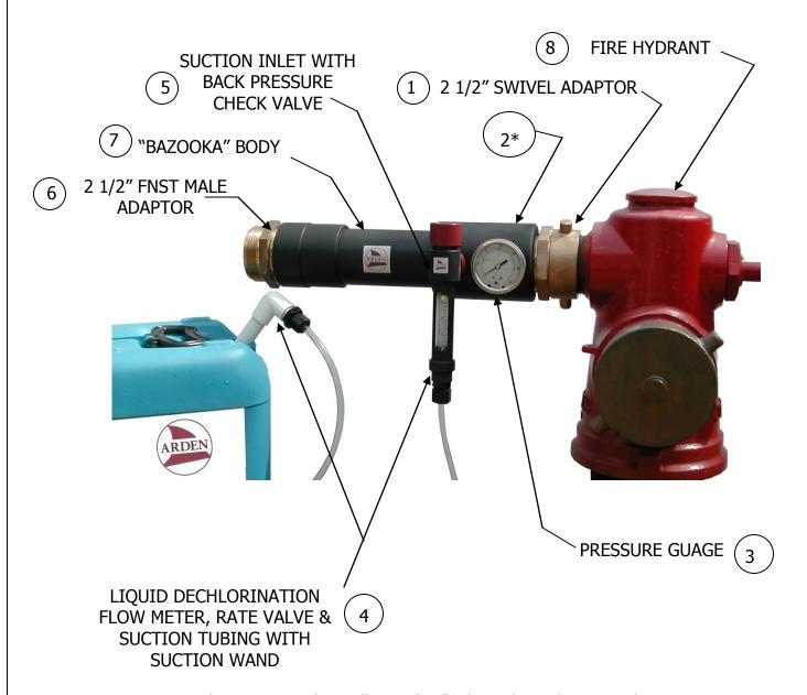
NOTE: 1. This is a typical installation for flushing through Fire Hydrants. Units can also be attached to 2-2 1/2" Risers from Water Mains for flushing super chlorinated water.
