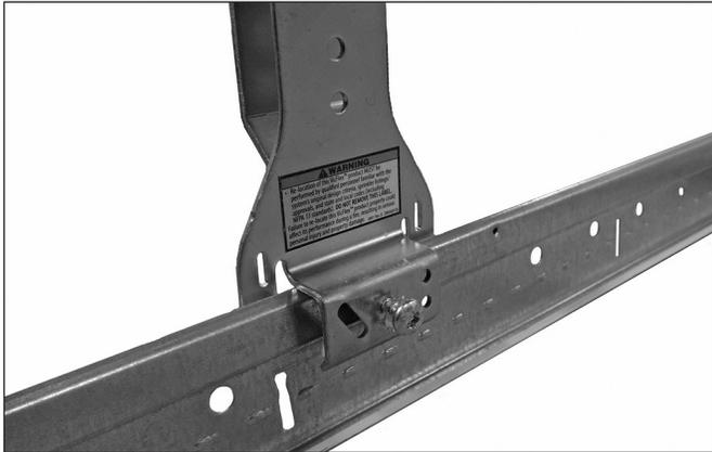
1. Attach the end brackets of the Style AB1, AB2, or AB10 Bracket to the T-bar rails of an ASTM C635 ceiling suspension system installed in accordance with ASTM C636 standards. Verify that the ends of the Style AB1, AB2, or AB10 Bracket engage the rails.
