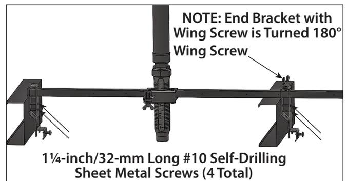
3. Rotate the end bracket assembly (side with the wing screw removed in step 2) 180°, as shown in the graphic above. Reinstall the wing screw loosely into the top of the end bracket assembly.
