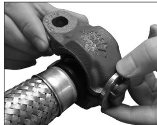
9. Install the linkage onto the housings, as shown to the left.
