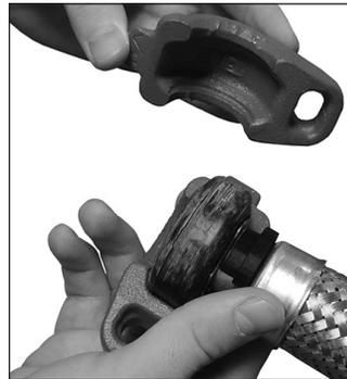
8. Place the lubricated gasket onto the inlet end of the flexible hose, then place the Style 108 Coupling housings over the gasket. Verify that the gasket is seated fully in the gasket pocket of each housing and that the housings' keys engage with the spacer.
