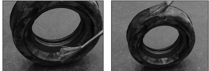
7. Apply a thin coat of a compatible lubricant, such as Victaulic Lubricant or an EPDM-compatible lubricant, to the gasket sealing lips and exterior. Silicone grease may be used (silicone spray is not a compatible lubricant). It is normal for the gasket to have a hazy white appearance after it has been in service.
