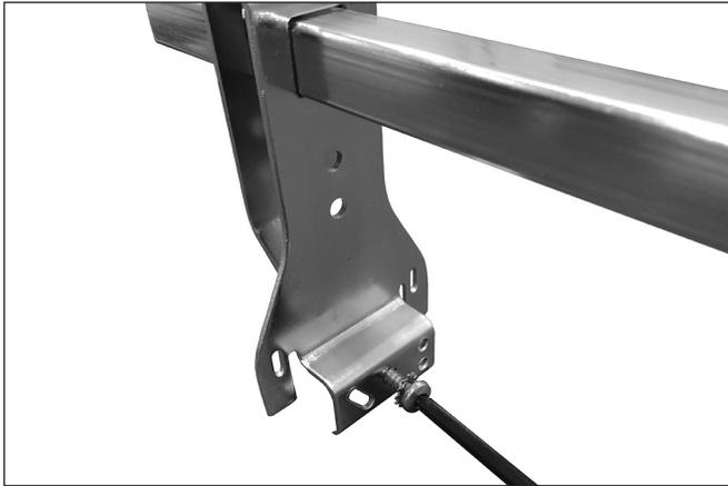
1. Using a T25 drive bit, remove the pre-installed sheet metal screw from each Style AB2 end bracket.
