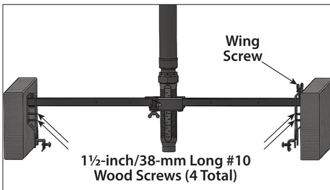
3. Place the end bracket assembly (without the wing screw) against the inside surface of the one wood joist/stud with the square bar resting on top of the wood joist/stud, as shown in the graphic above.
