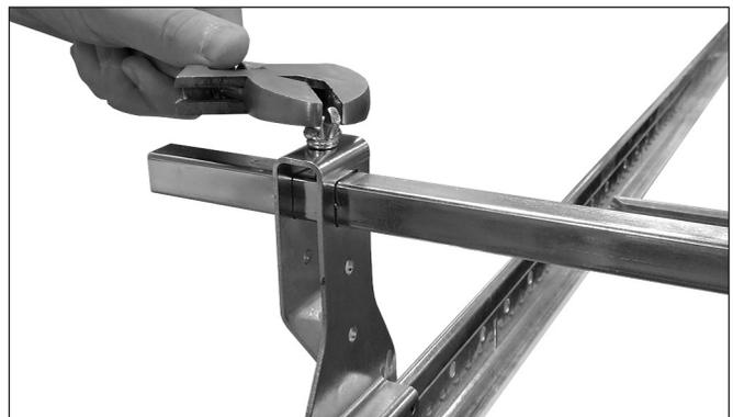
**FOR STYLES AB1 AND AB2 BRACKETS ONLY:** Verify that the wing screw on top of the end bracket assembly is tightened to a torque of 36 inch-lbs/4 N•m (approximately ½ to ¾ of a turn past hand-tight).
