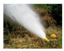
NOTE: Many operators actually use the Shut-Off Gate Valve to conduct the flow procedure to avoid water hammer during throttling down of the flow. This reduces wear on the hydrant and allows you to fully open the hydrant's main valve and reduce the chance of debris infiltration. Note in some cases putting a Hydrant Slow close Gate Valve in front of the HydrantPro can cause turbulence and prevent accurate readings on the flow gauge.
