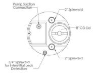
Typical top configuration. Some sizes vary. Full drawing details available on etanks.com **Wide Range of Sizes**
