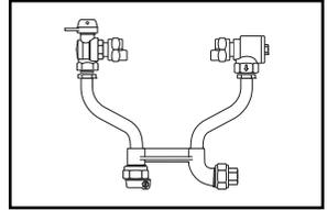
**ANGLE BALL VALVE BY ANGLE DUAL CHECK VALVE (5/8"x3/4" METER)**
