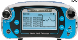
The "Saved" data file showing 10 leak sound levels and graphical display. Leak is at the peak sound level in the center.
