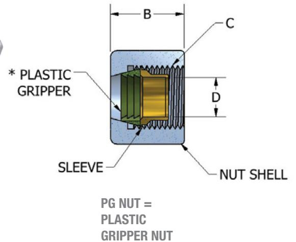
\*Note: P/K Material Nut: Use PVDF Material Gripper, N/C Material Nut: Use Acetal Copolymer Gripper
