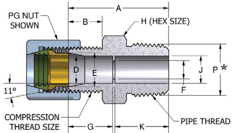
Section shown with Nut Style, PG, Plastic Gripper Nut
