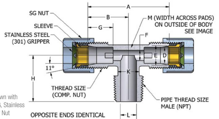
Diagram shown with Nut Style, SG, Stainless Steel Gripper Nut
