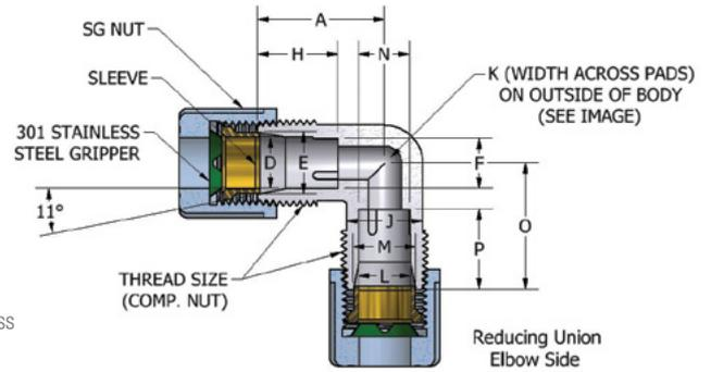
Diagram shown with Nut Style, SG, Stainless Steel Gripper Nut
