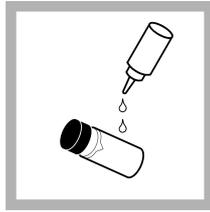
2. Wipe with lint-free cloth. Apply a thin film of silicone oil (Apply silicone oil to a sample cell on page 20).
