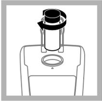
7. Remove the cell, rotate it slightly approximately  $\frac{1}{8}$  of a turn and insert it again into the cell compartment. Close the lid.
