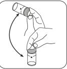
Dissolve tablet(s) by inverting.
