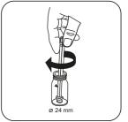
Crush tablet(s) by rotating slightly.
