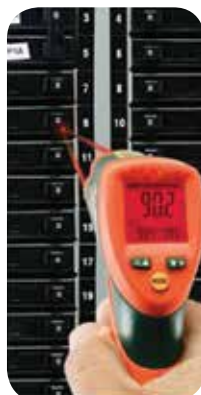
Red backlight plus audible alert: exceeds temperature
