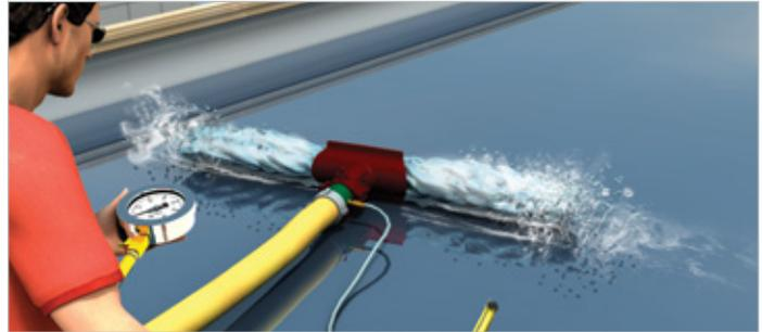
The Little Hose Monster and Pitotless Nozzle in a rooftop standpipe test.
