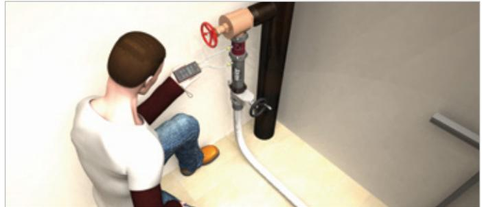
The In-line Pitotless Nozzle in a stairwell standpipe test.
