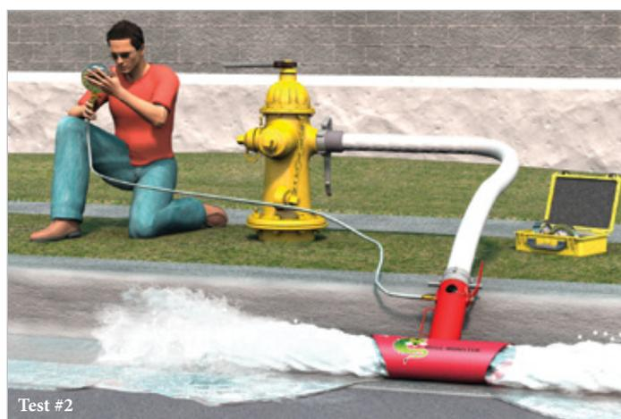
In summary, the test flows will be different, but the difference will not affect the flow test. The Hose Monster and hose will result in a lower test flow-rate and a higher residual pressure. When all data is considered, the flow tests result in the same predicted flow-rates.
