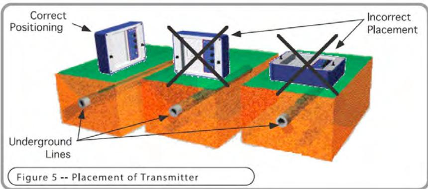
If the transmitter is aligned perfectly with the underground line, the signals emerging from the sides will travel along the path of the line. This can cause some confusion when working close to the transmitter. To avoid such confusion, offset the transmitter  $10^\circ$  or  $15^\circ$  from the general direction
