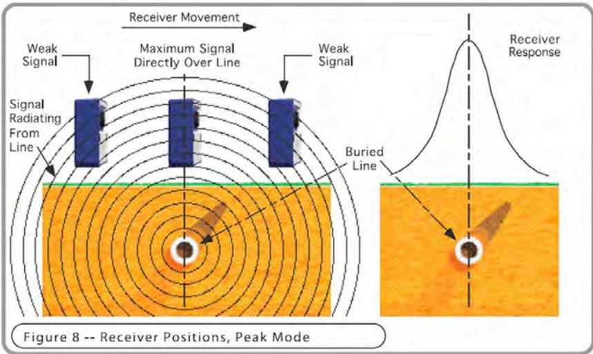
iv) Now move the receiver back and forth, causing the meter and sound response to increase and decrease and "peak" over the line. Continue peaking over the line as you walk in the direction of the line; the line will be directly below where the signal response is maximum as you walk.
