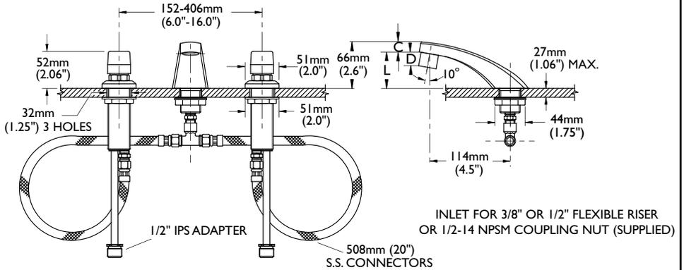
INLET FOR 3/8" OR 1/2" FLEXIBLE RISER OR 1/2-14 NPSM COUPLING NUT (SUPPLIED)
