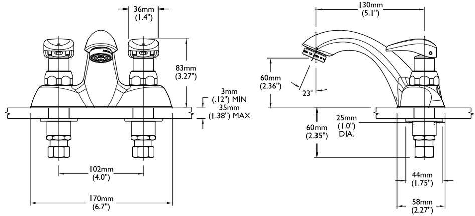
INLET FOR 3/8" OR 1/2" FLEXIBLE RISER OR 1/2-14 NPSM COUPLING NUT (SUPPLIED)
