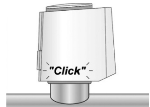
3. Press down vertically and snap the actuator onto the adapter ring.
