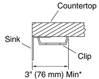
\* Allow clearance around sink rim for clip attachment.
