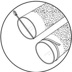
Measure the pipe's Outer Diameter and make sure the coupling's size fits properly.
