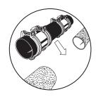
Slide the two HYMAX GRIPs on both sides the replacement pipe. (according to the application - for example, one HYMAX Grip Flange adaptor and one HYMAX Grip coupling) Lower the replacement pipe and the two grips positioned on it into the ditch.
