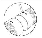
Mark each pipe end to a minimum required stab depth as indicated on the product label. These marks indicate the required stab depth of the pipe on the coupling.
