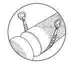
Prepare both pipe ends of the pipe by de-scaling if required. Clean the pipe as required with water. Make sure that the pipe is clean from debris and defects that interfere with HYMAX's proper seal.
