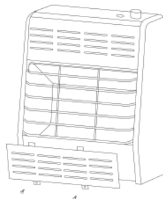
Figure 6 - Removing Lower Front Panel Of Heater
