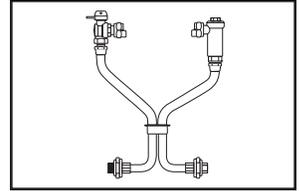
ANGLE BALL VALVE BY ANGLE DUAL CARTRIDGE CHECK VALVE (5/8" X 3/4" METER)
