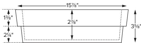
NOTES: SINK IS SEMI-RECESSED. SINK MUST BE MEASURED ON-SITE TO ENSURE ACCURATE DIMENSIONS OF HOLE CUT-OUT.
