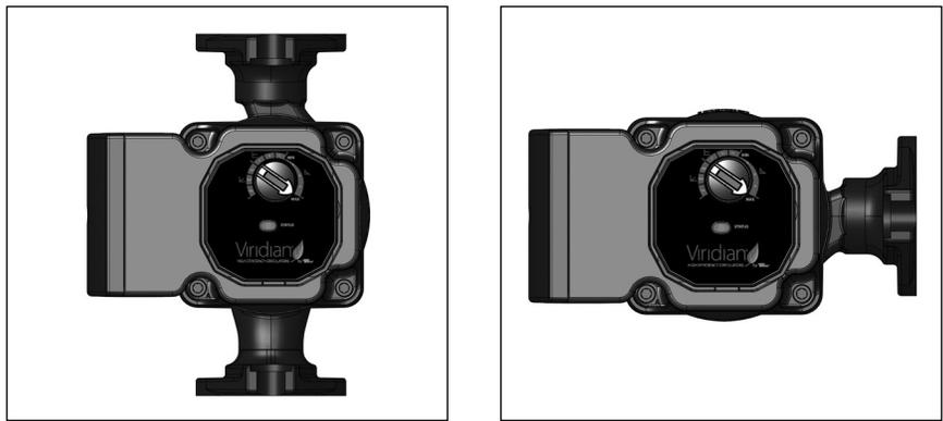
Position electrical junction box at 9 o'clock position for best programming and viewing orientation. Casing may be rotated to change flow direction. Locate the arrow on the casing body to determine flow direction.
