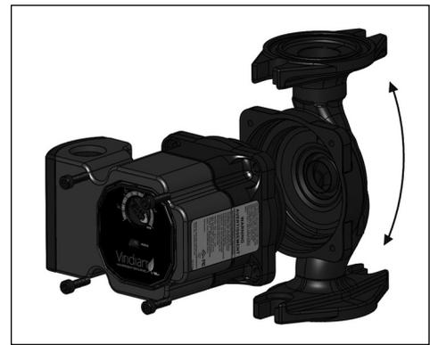
To rotate the casing, remove the 4 motor screws and spin the casing to the desired flow direction. Reattach the 4 screws (5/32" allen wrench required). Be sure body gasket is seated evenly to prevent leakage. Tighten motor screws to 34-42 in-lbs torque.
