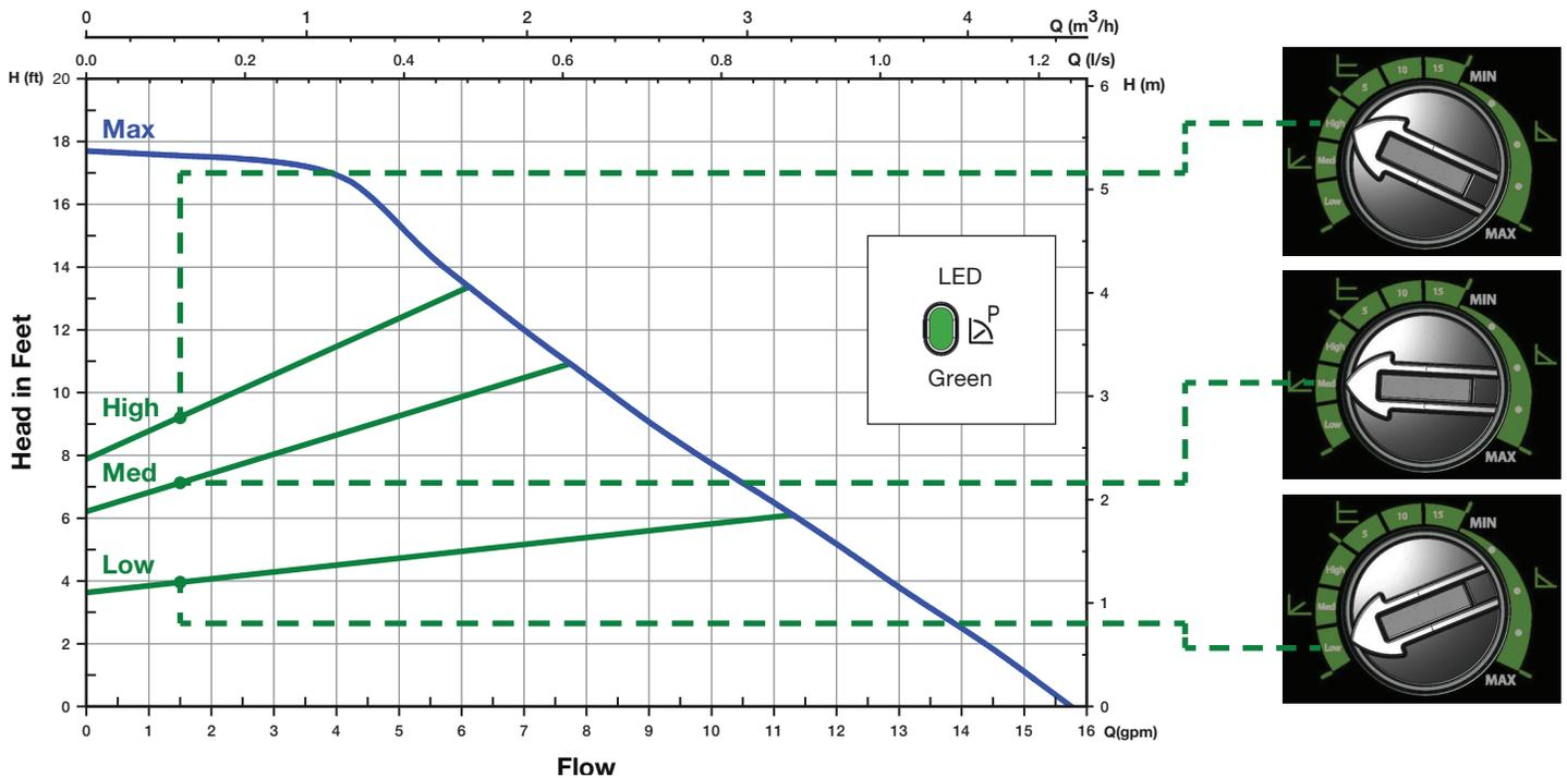
In Proportional/variable pressure mode (∟), the circulator maintains a proportional pressure differential ( $\Delta p-v$ ) as heating load increases or decreases. Flow will change in relationship to the change in pressure differential. Selection options are Low, Medium, or High. If unsure on proper setting, select Medium and adjust as needed.
