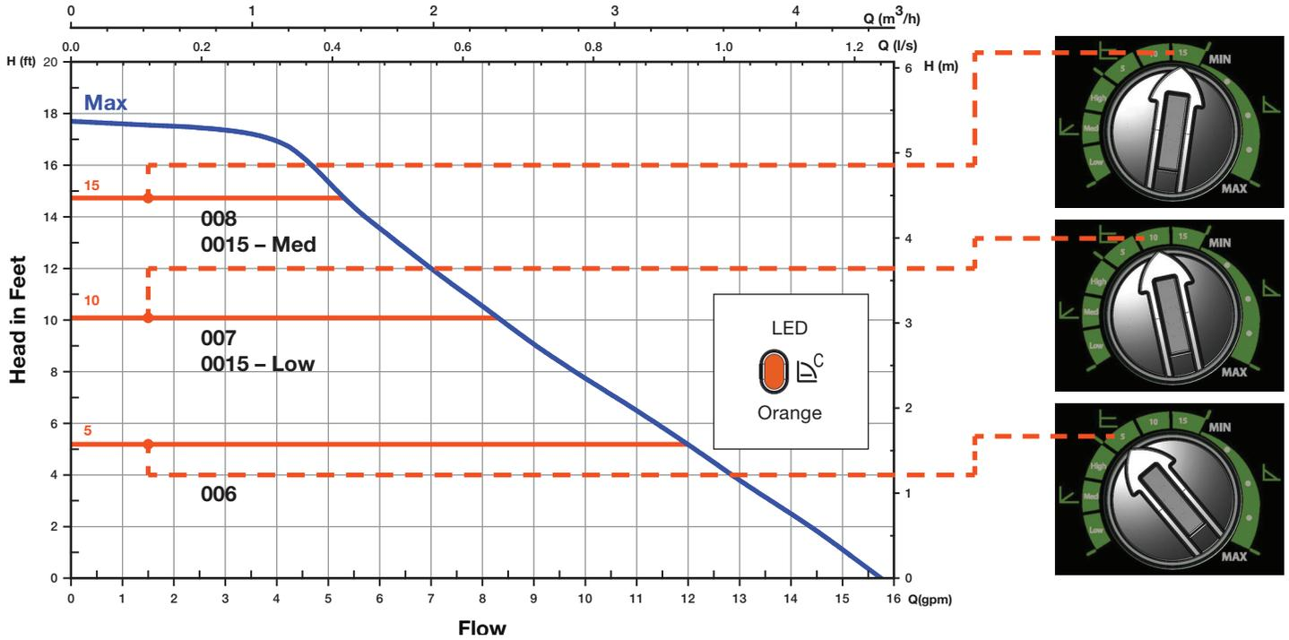
In Constant pressure mode (⊥), the circulator maintains a constant pressure differential ( $\Delta p-c$ ) in the system as heating load increases or decreases. Selection options are 5, 10, or 15 feet of head constant pressure. See chart above for equivalent 00 model at each setting.
