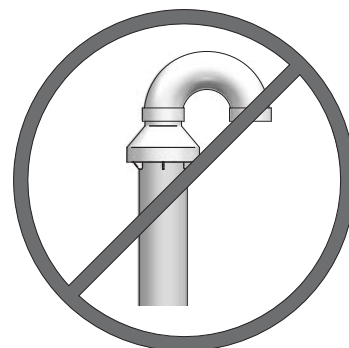
Figure 5-5 Do Not Install U-Bend to Rain Cap
